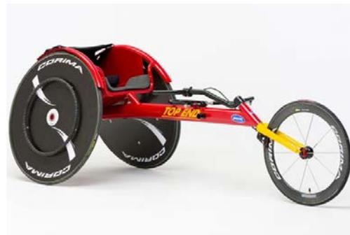
**Racing:** lightweight, carbon wheels, no casters, long front end, steering system, no foot plate, small push rims
